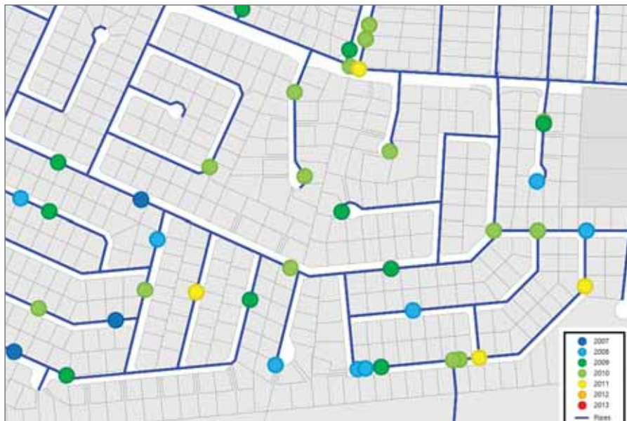
Figure 1: Historic incidents of pipe failures on top of the network layout
