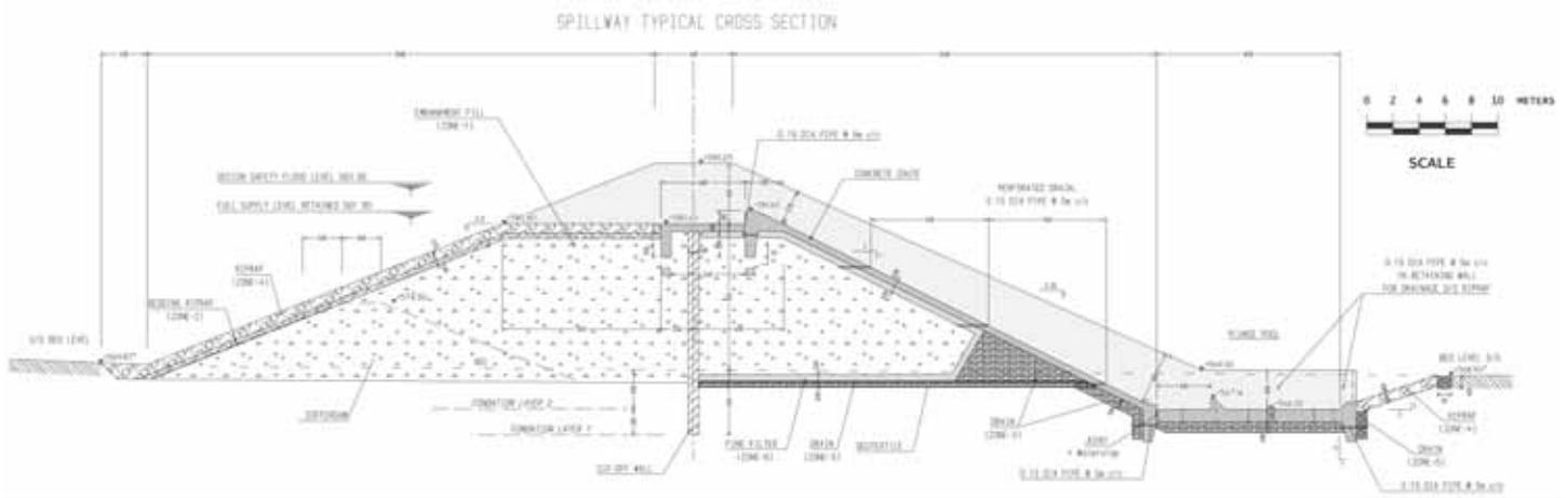
**Cross section of the 18 m high Wadi Kalboh Dam in Oman, a groundwater recharge dam**
