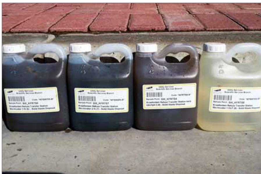
Figure 11 Visual contrast between influent and effluent SW samples (April 2013)
