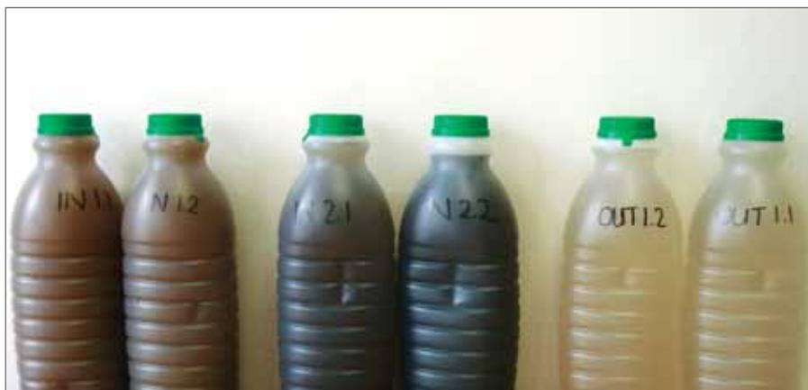
Figure 10 Visual contrast between influent and effluent SW samples (April 2012)
