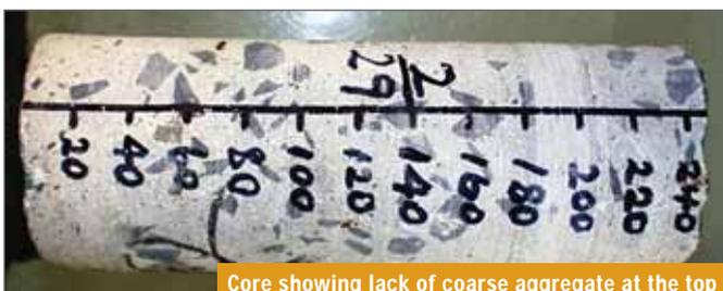
Core showing lack of coarse aggregate at the top
