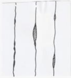
d. Reinforcement Corrosion
