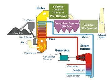
Supercritical technology and its advantages - In other words, supercritical power plants are highly efficient plants with best available pollution control technology, reduces existing pollution levels by burning less coal per megawatt-hour produced, capturing the vast majority of the pollutants. This increases the kWh produced per kg of coal burned, with fewer emissions.
