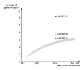
"Supercritical" is a thermodynamic expression describing the state of a substance where there is no clear distinction between the liquid and the gaseous phase (i.e. they are a homogenous fluid). Water reaches this state at a pressure above 22.1 MPa. The efficiency of the thermodynamic process of a coal-
