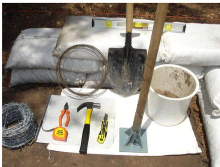
Inexpensive materials form earthbag walls. Grain bags are filled with moist earth, stacked, tamped, and covered with plaster. Under roofs they dry into an improved adobe with tensile strength from fabric, barbed wire, and mesh.
