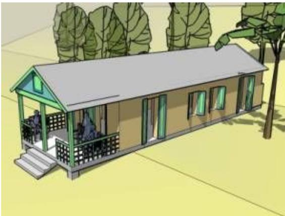
A kay is a long, narrow building (like the shotgun houses in the US which probably developed from it). Each room opens into the next without any hallways, allowing good cross-ventilation. It is easy to add onto, by extending the same rooflines. By adding a shallower roof onto one side it can become an L shape.
