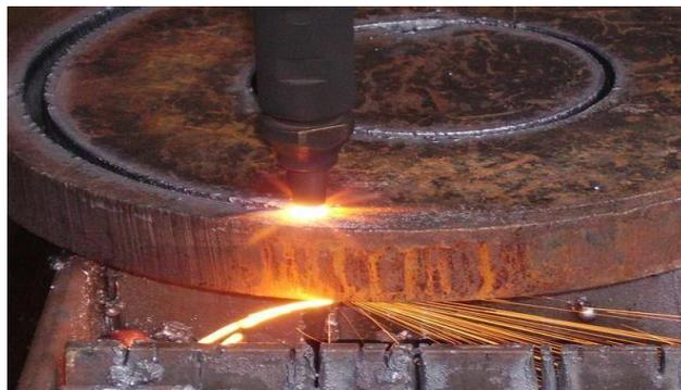
These systems can easily cut ferrous materials for more than 200 mm (8 inches) and is a one of the preferred tools for manual cutting of thick steel (more than 38 mm or 1 ½ “),
