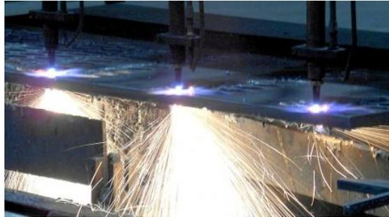
The “oxyfuel” system is an auxiliary technique to welding developed since 1903 and used to date in many industrial applications.
