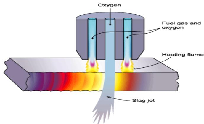
In the presence of oxygen at high temperatures focused, an exothermic oxidation occurs in the iron which supplies all the heat required to “burn” it, transforming it into ferric oxide ( $\text{Fe}_2\text{O}_3$ ), which melts in the form of sparks because its melting is lower than that of steel or is blown across the surface.
