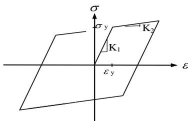
Fig. 3 Bilinear spring model
