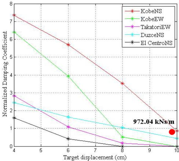
Fig. 5 Normalized damping coefficient vs. target displacement for longitudinal (top) and transverse (bottom) axis
