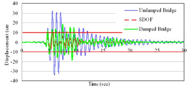
Fig. 7 Displacement time response for the midspan under transversal Kobe-NS earthquake
