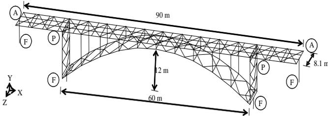
Fig. 2 Configuration of three-dimensional finite element model
