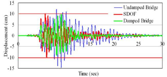
Fig. 6 Displacement time response for the deck under longitudinal Kobe-NS earthquake
