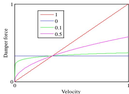
Fig. 1 Damper force-velocity relationship
