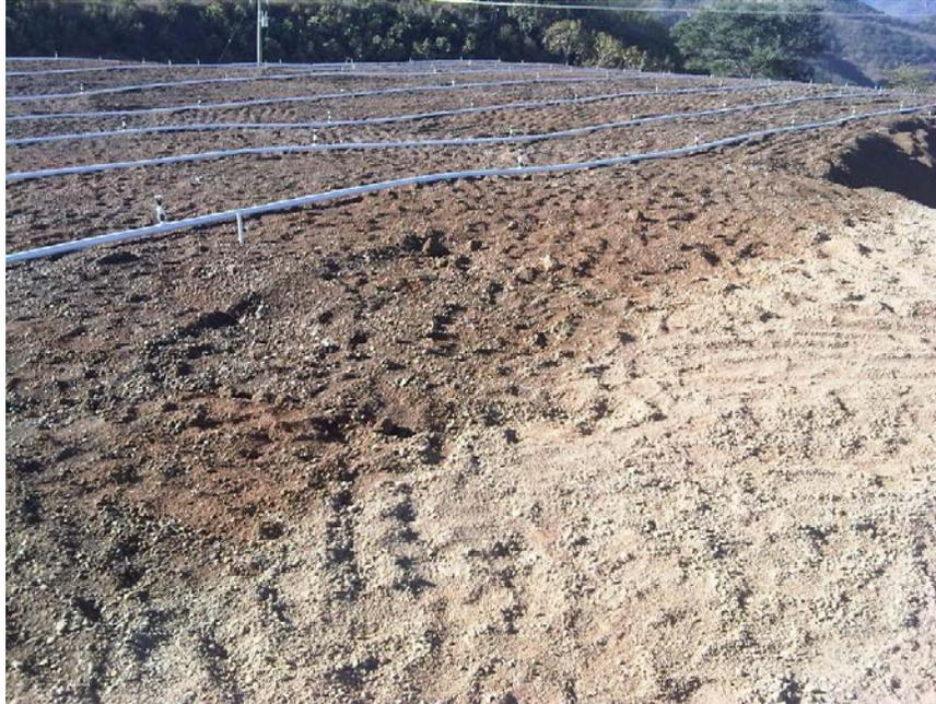
Compared to pyrometallurgical operations, leaching is a much simpler and much less harmful because gaseous pollution never occurs, and because its energy consumption is very low, mostly depending on gravity's action and pumping solutions to the heap.
