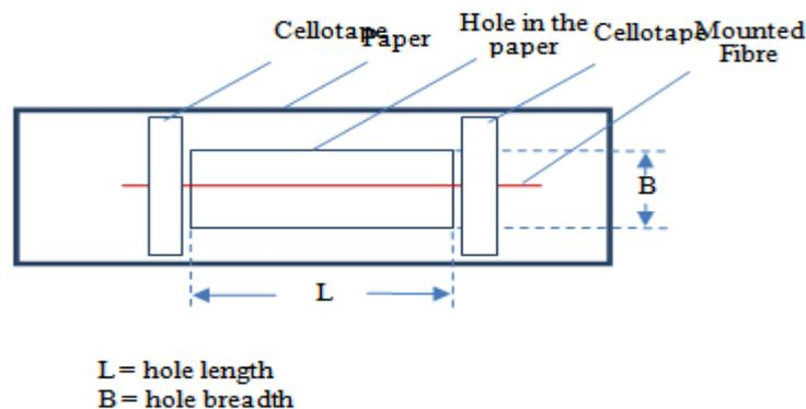
**Figure 3: Test sample preparation**
