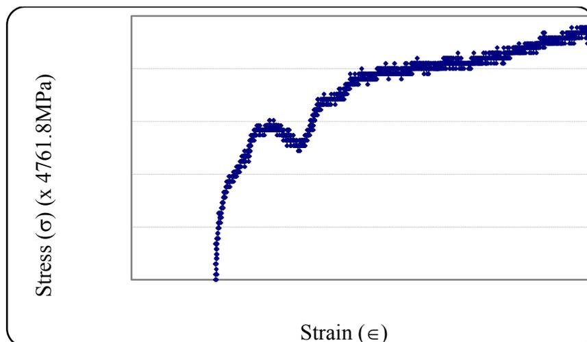
Figure 7 Alpaca fibre's behaviour under continuous loading
