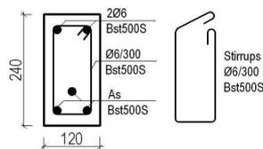
Fig. 2 Cross section
