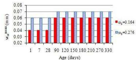
Fig. 5 Mean experimental values of cracks widths
