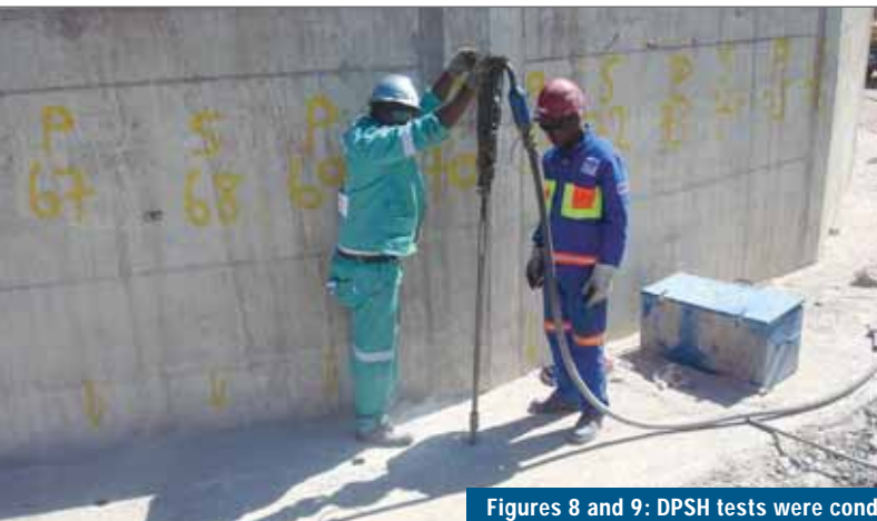
Figures 8 and 9: DPSH tests were conducted to assess in-situ soil consistency
