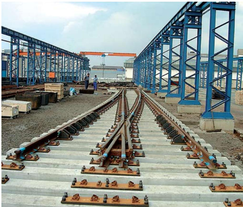
► The first 1 in 9 turnout set manufactured by VAE South Africa for the Gautrain Rapid Rail Link project shortly before delivery to the Gautrain Sleeper Joint Venture. The set was assembled using highly specialised concrete sleepers manufactured to a tolerance of 0,25 mm by Infraset Infrastructure Products
