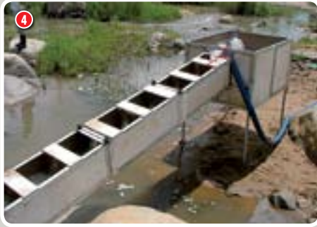
1 A 1:1 scale prototype double fishway channel was built and tested under various flow conditions at the Hydrometrics Laboratories, DWAF, Pretoria. Various fish species were used during the testing to determine the success rate of such a channel 2 Fish congregate en masse at migratory barriers during the high-flow summer season (Kruger Gate weir, Sabie River, KNP, November, 2004). Only a relatively small percentage of these individuals will successfully negotiate the barrier to utilise upstream habitats for reproduction, genetic dispersal and habitat exploitation. Many
