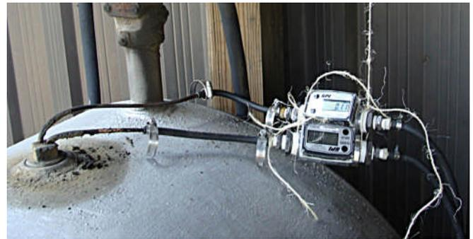
Figure 5 Flow meters and fuel tank providing fuel to compressor engine
