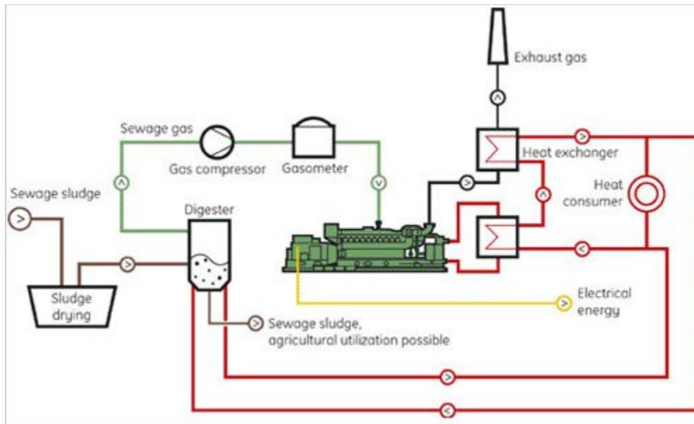
Sewage gas is harvested in much the same way. Sewage sludge is first dried and then pumped into a digester. The gas emitted from the digester typically contains about 50 to 60% methane. The gaseous emissions are then compressed and fed to a gasometer. This acts a fuel tank to the actual electrical energy generator unit. Enough energy is generated to power the sewage treatment plant itself.
