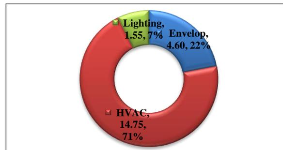
Figure 7: Effect of building envelop, HVAC system and lighting system related EEMs in percentage savings of annual energy consumption
