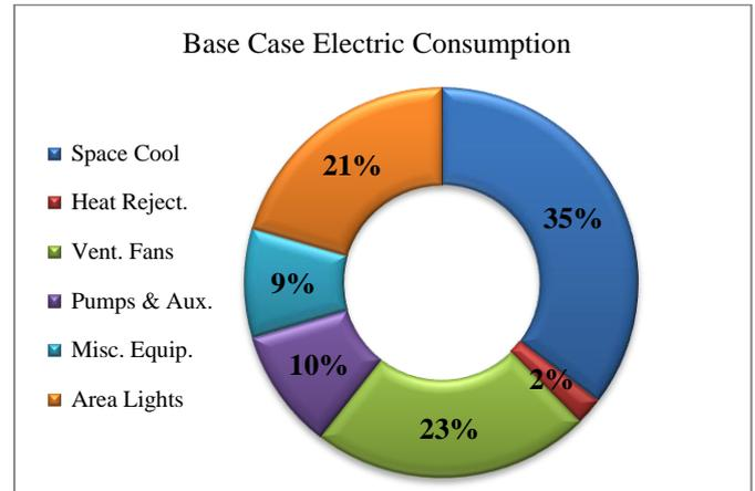
Figure 4: Base case energy consumption breakdown in percentage
