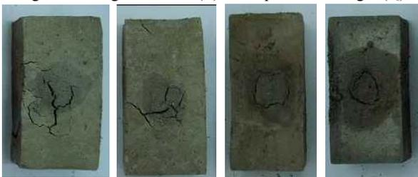
Non-baked specimens: severely damaged during tests
