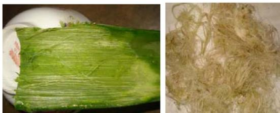
Fig. 1 Pineapple leaf fibres, PF: raw (left) and dried (right)
