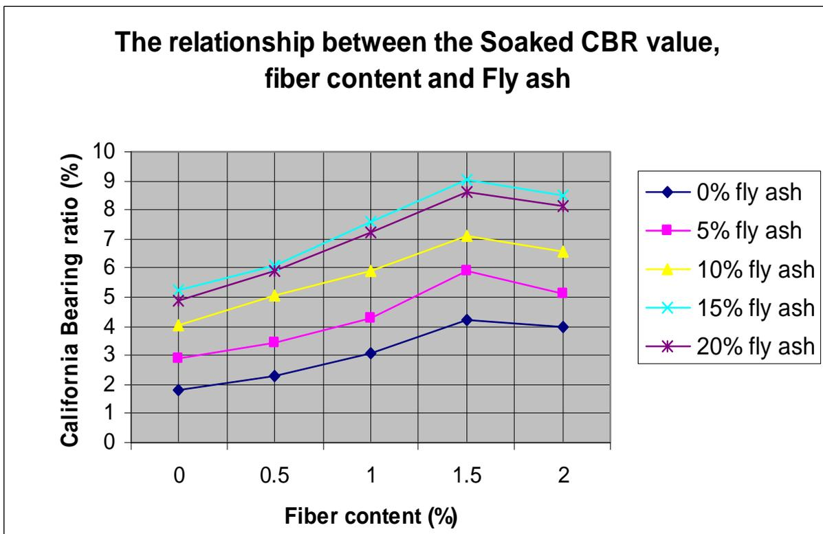
Graph-2, Variation of CBR for soaked condition with and without addition of fibers to the fly ash Soil
