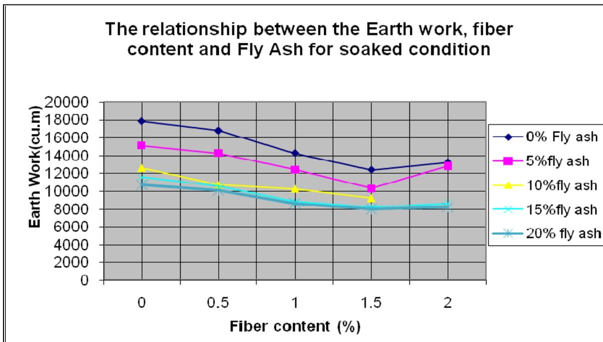
Graph 6: The relationship between the earth work, fiber content and fly ash for soaked condition
