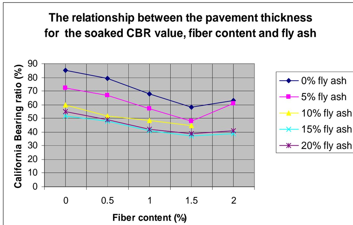
Graph-4, Variation of thickness of pavement for soaked condition with and without addition of fibers to the fly ash Soil
