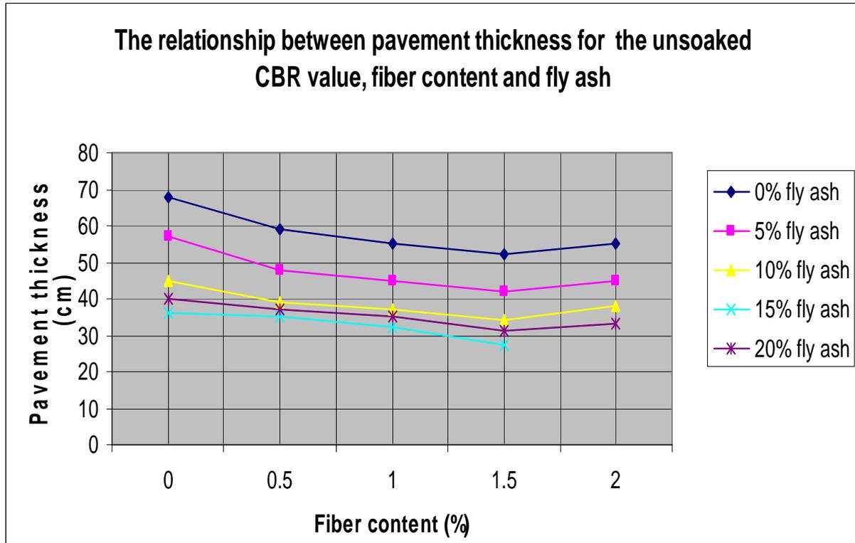
Graph-3, Variation of thickness of pavement for un soaked condition with and without addition of fibers to the fly ash Soil
