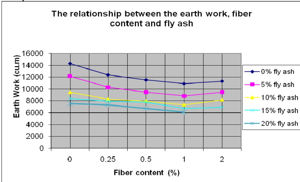
Graph:5 The relationship between the earth work, fiber content and fly ash for unsoaked condition
