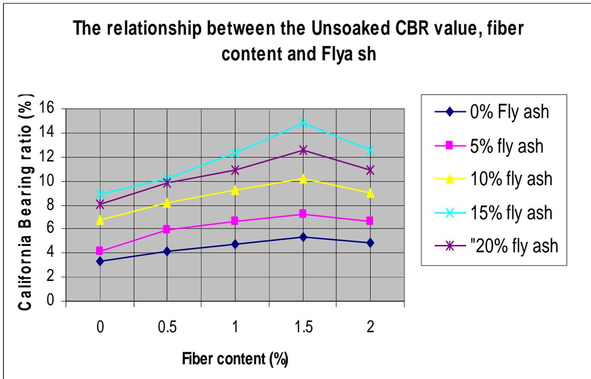
Graph-1, Variation of CBR for un soaked condition with and without addition of fibers to the fly ash Soil
