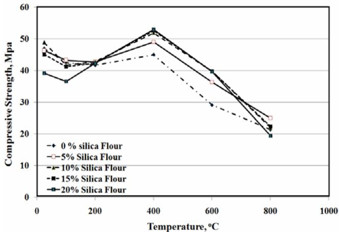
Fig. 1. Compressive strength of concrete exposed to elevated temperature after cooling
