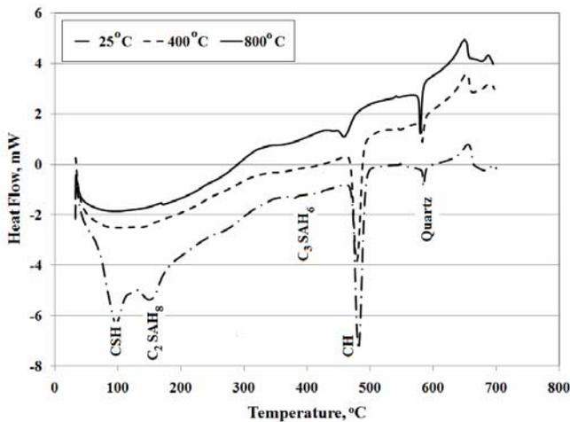
Fig. 4. DSC thermograms of silica flour concrete thermally treated at 25, 400 and 800°C
