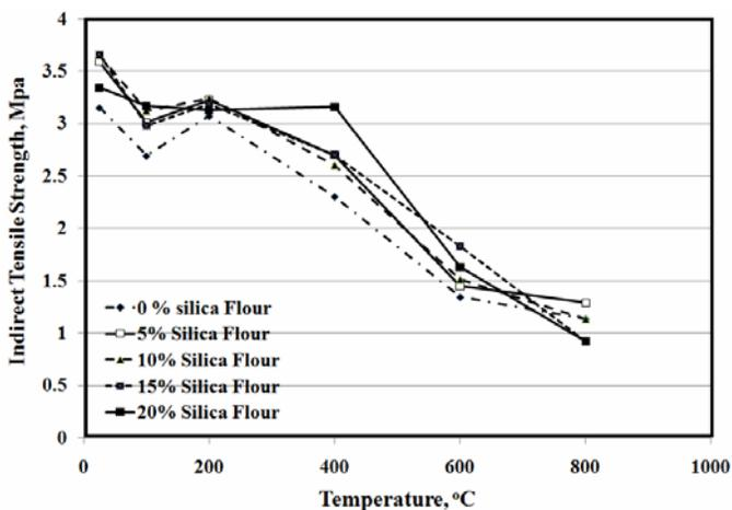
Fig. 2. Indirect tensile strength of concrete exposed to elevated temperature after cooling
