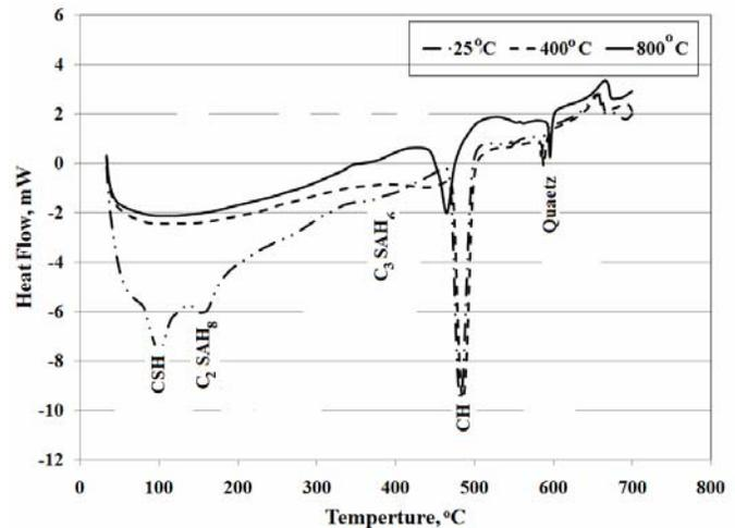
Fig.3. DSC thermograms of control concrete thermally treated at 25, 400 and 800°C
