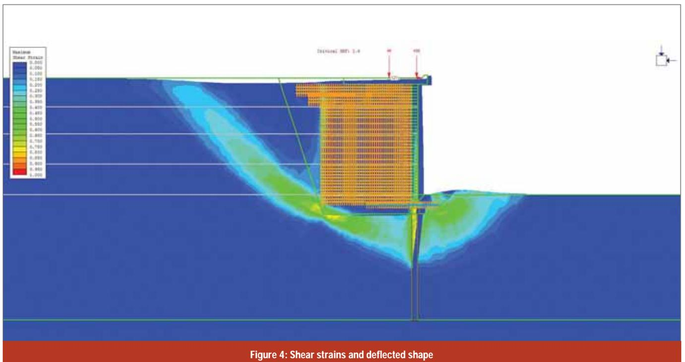
Figure 4: Shear strains and deflected shape
