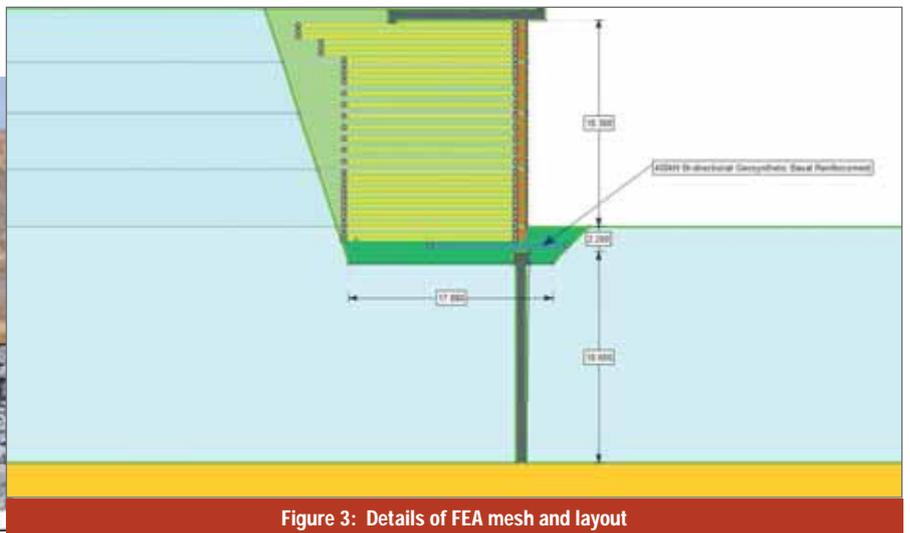
Figure 3: Details of FEA mesh and layout
