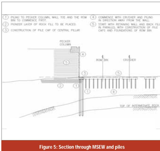
Figure 5: Section through MSEW and piles
