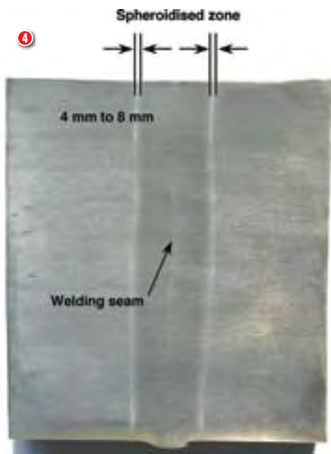
► Figure 4 Cross-section showing the spheroidised zone
