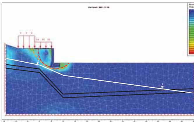
**Figure 7** FEM SSR slope stability results – after demolition, but before excavation
