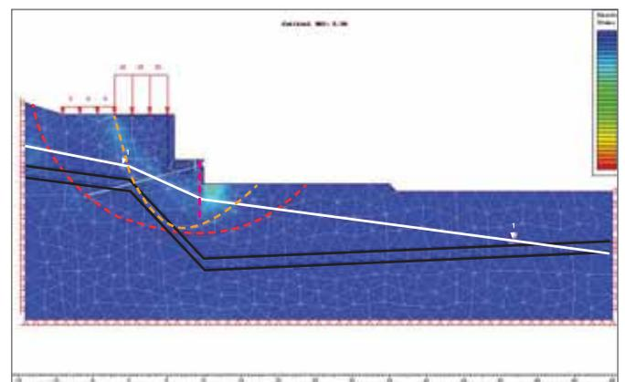
**Figure 8** FEM SSR slope stability results – after excavation
