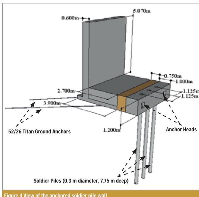
Figure 4 View of the anchored soldier pile wall
