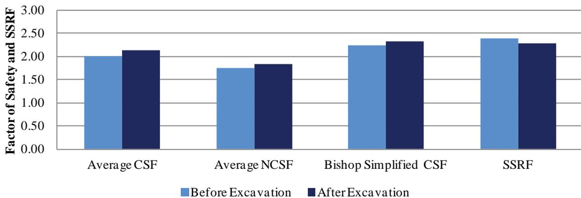
**Figure 6** Comparison of slope stability results
