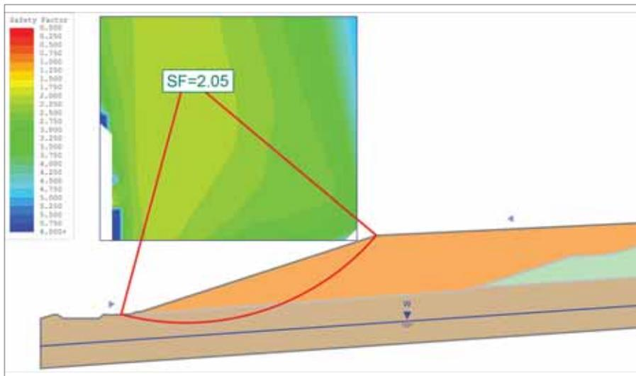
Figure 3: Slope 2 - LE analysis (circular slip surface)
