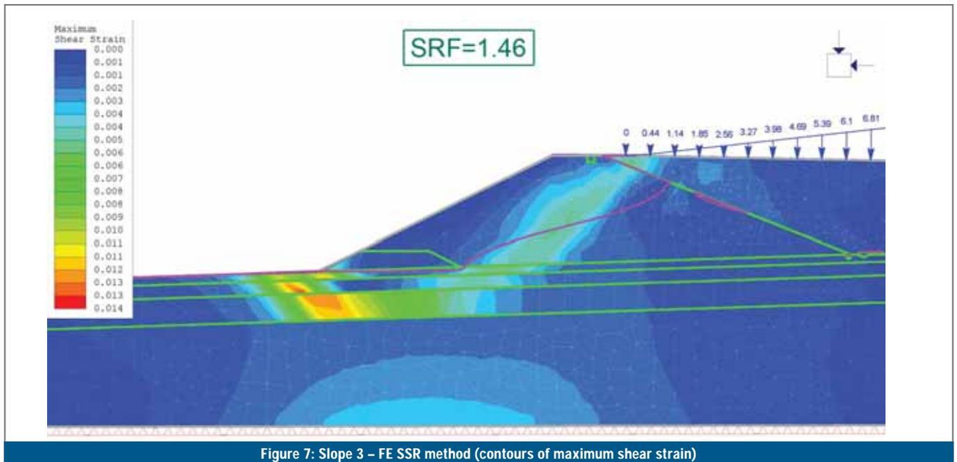
Figure 7: Slope 3 – FE SSR method (contours of maximum shear strain)
