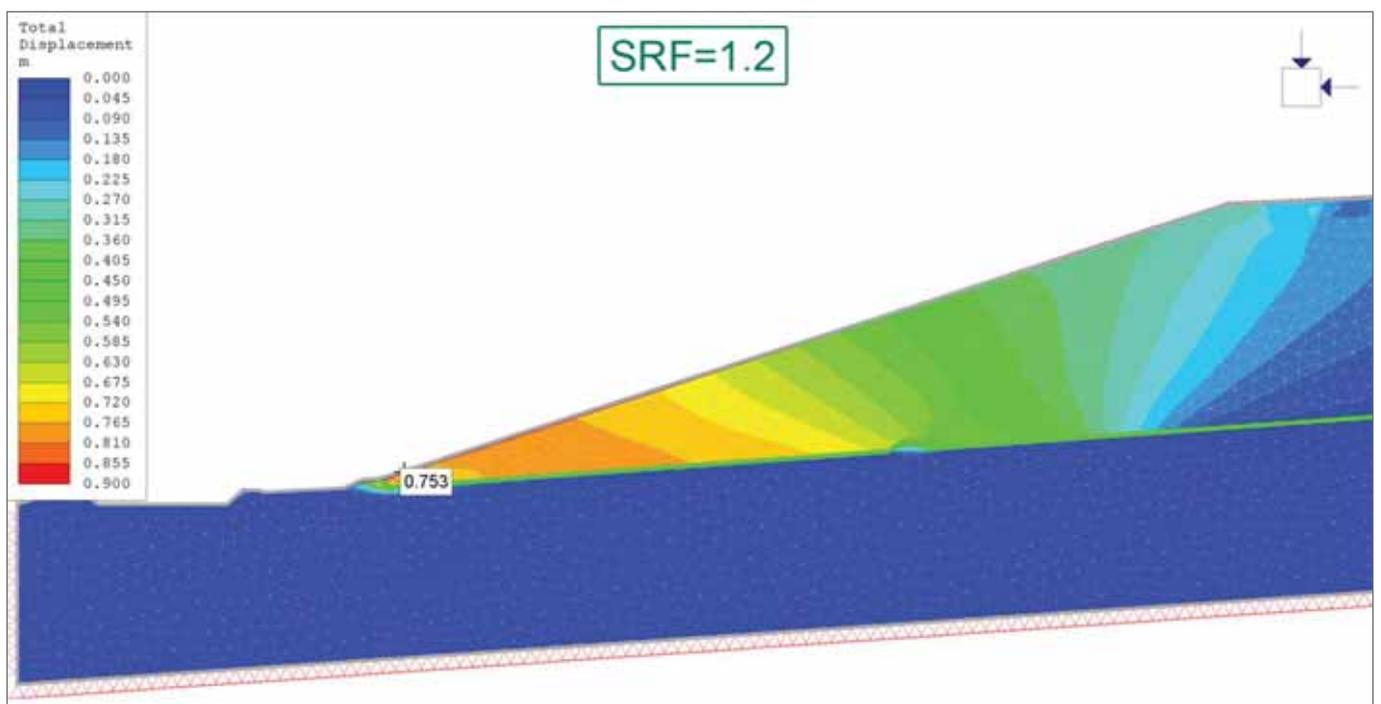
Figure 5: Slope 2 - FE SSR method (contours of total displacement)
