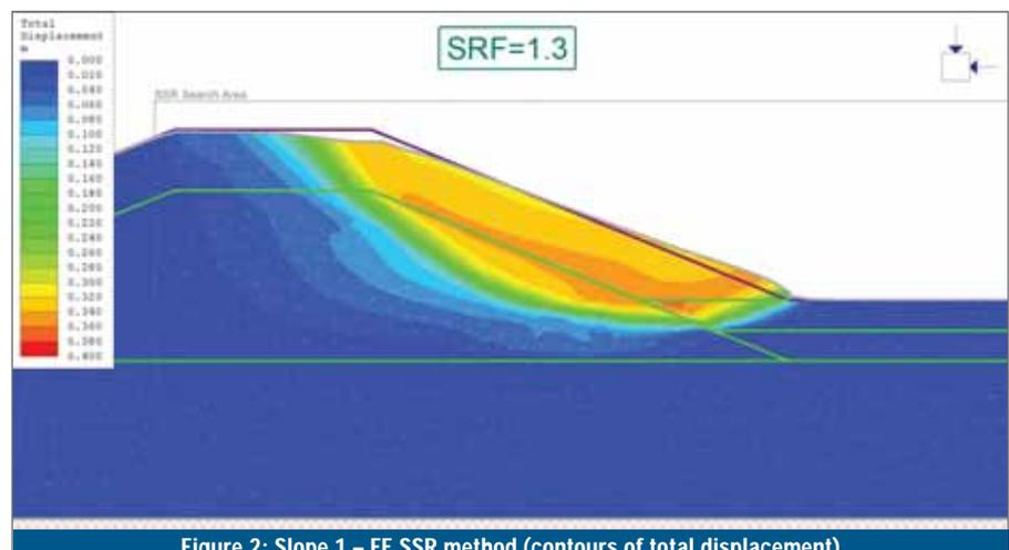
Figure 2: Slope 1 – FE SSR method (contours of total displacement)
