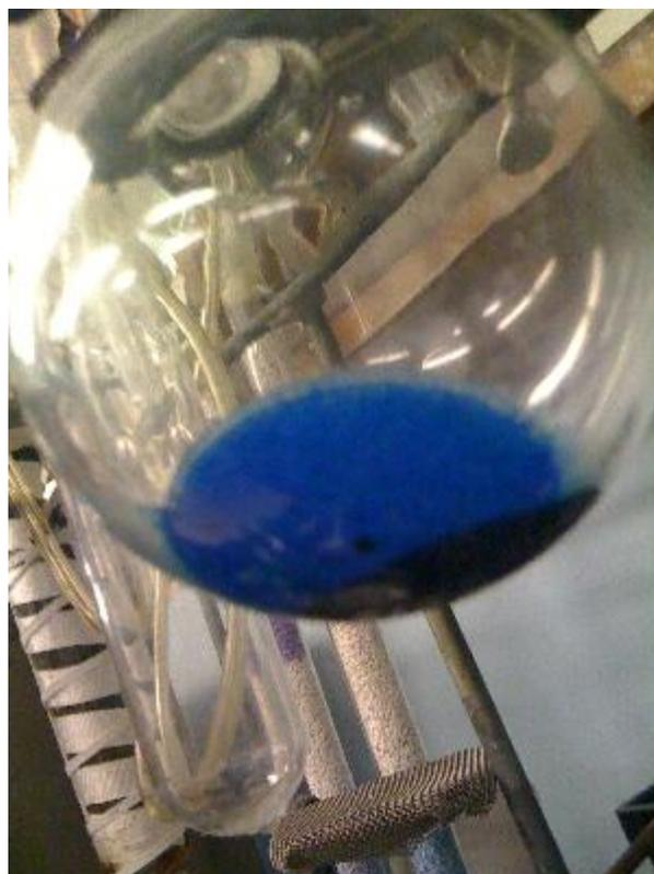
**Figure x: Organometallic chromium crystals in a Schlenk under nitrogen**
