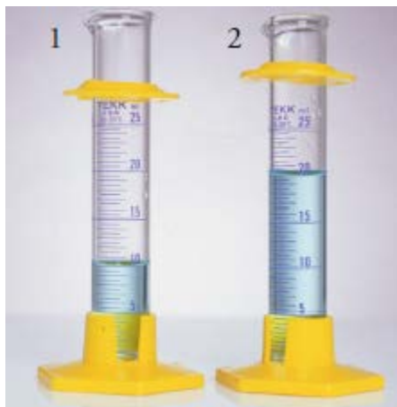
Figure 3.3 Graduated cylinders containing 0.010 M \text{Cu}(\text{NO}_3)_2 . Although the cylinders contain the same concentration of \text{Cu}^{2+} , the cylinder on the left contains 1.0 \times 10^{-4} mol \text{Cu}^{2+} and the cylinder on the right contains 2.0 \times 10^{-4} mol \text{Cu}^{2+} .
