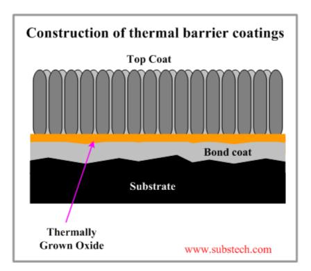
■ Metallic Bond Coat with a thickness of about 0.004" (0.1 mm). The alloy of the bond coating is MCrAIY, where M is Ni, Fe or Co. The bond coat is an intermediate layer providing strong adhesion of the outer ceramic layer to the substrate surface. The bond coat also inhibits the diffusion of the substrate and the ceramic coating components. Aluminum in the amount of about 10% in the bond
