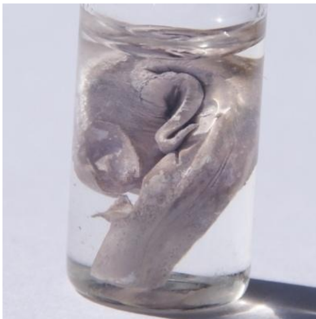
0.5 grams sodium with a white hydroxide (NaOH) crust under paraffin oil. Original size in cm: 1 x 1.5 . Source: images-of-elements.com
