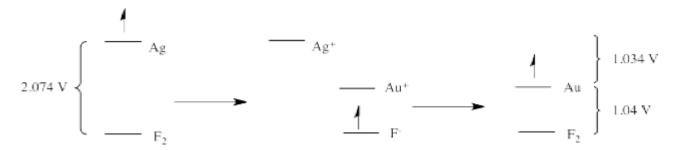
That's the same value we would expect to measure if we took a standard solution of gold salts and a gold electrode and connected it, via a circuit, to a standard solution of silver salts and a silver electrode.
