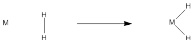
Figure OA2.1. Our general scheme for an oxidative addition of hydrogen to a metal.
