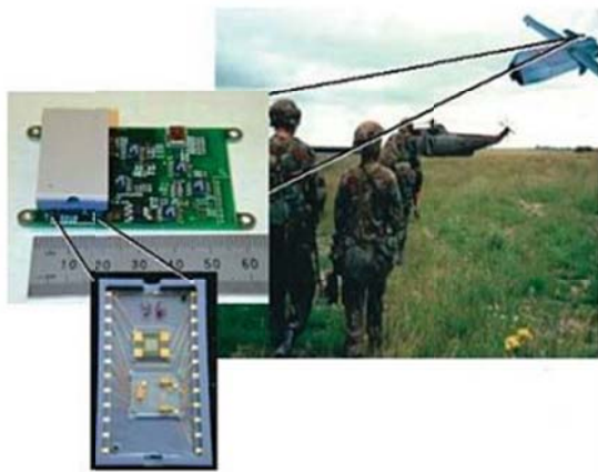
SnifferSTAR is a nano-enabled chemical sensor integrated into a micro unmanned aerial vehicle
