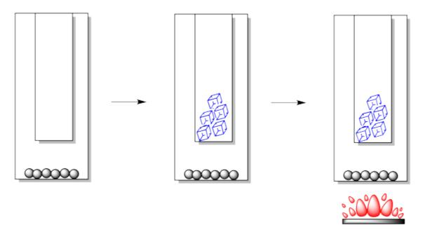
After the sample is heated for some time, crystals begin to form higher in the apparatus. Usually, they form on the cold finger, but they may also form higher up the walls of the outer vessel. The crystals may first appear in different forms or habits: they may be light and feathery, round and scaly, needles or blocks.
