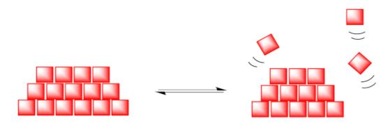
At lower temperatures, a solid material is expected to be crystalline and ordered. However, at higher temperatures, enough energy may be gained by the molecules in the solid so that they can escape into the gas phase.
