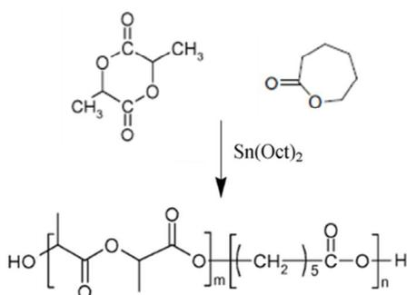
Fig. 1 Synthesis and structure of PLA/PCL biopolymers
