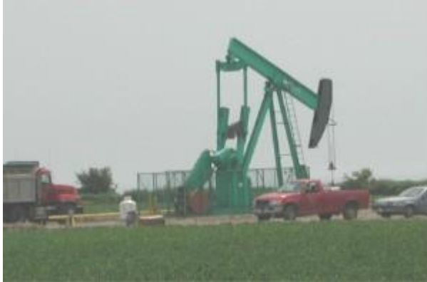
Pumpjack pumping an oil well near Sarnia, Ontario
