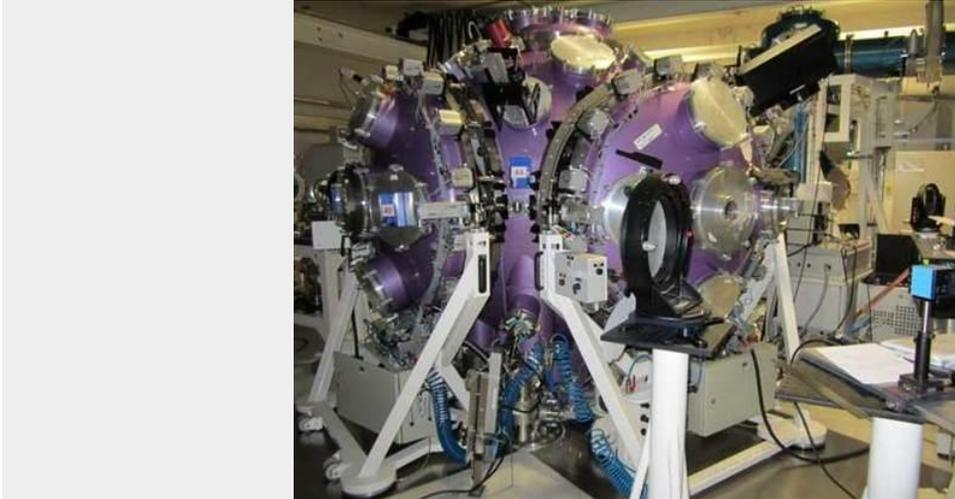
The experimental chamber in which the proton-boron fusion reactions were produced.
