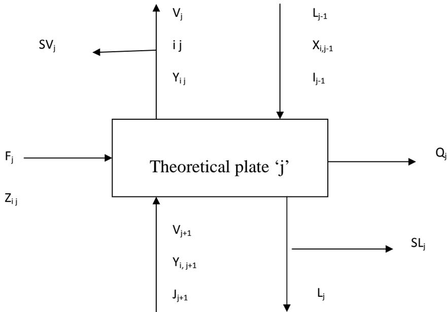
**Fig. 26.2:** Theoretical Plate of a Continuous Column
