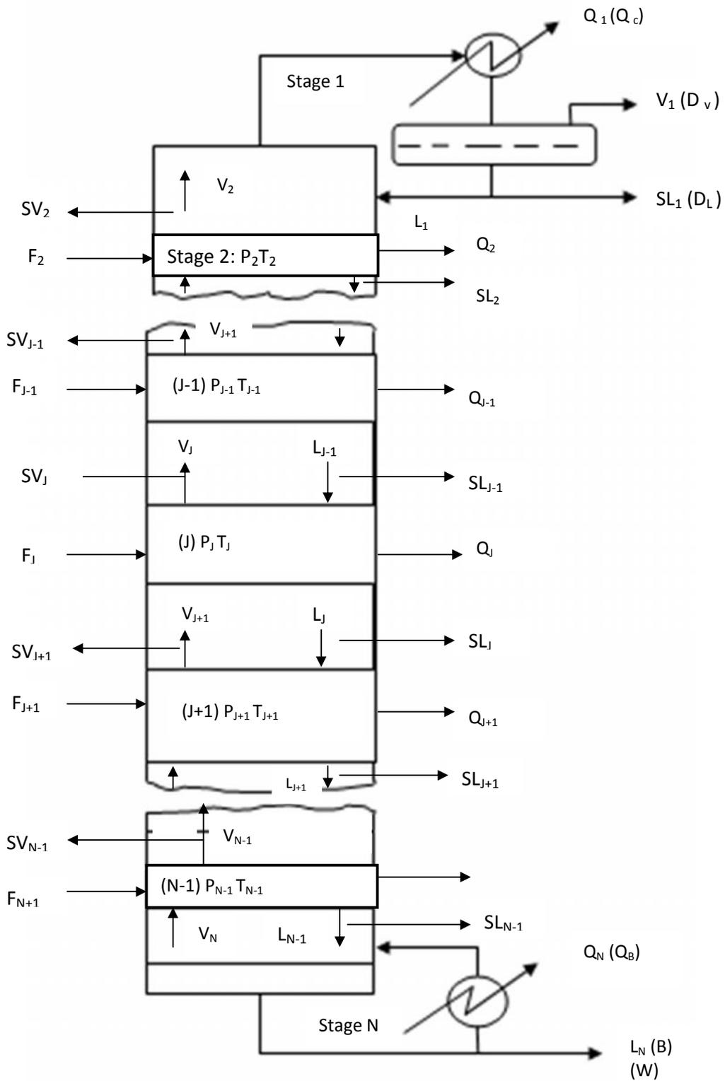
**Fig. 26.1:** Continuous Distillation Column
