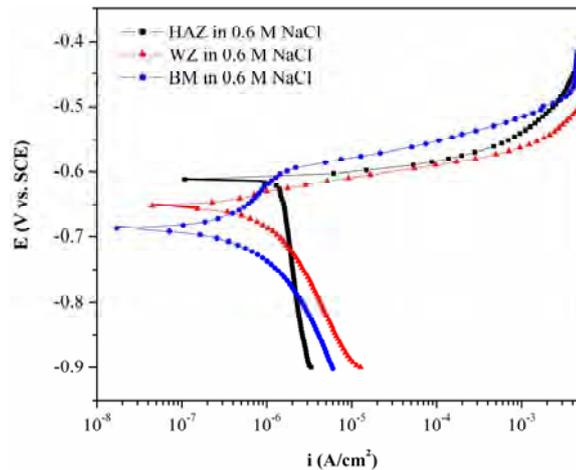
Fig.2. Potentiodynamic polarization curves for top surface AA2219-T87 welded plate in 0.6 M NaCl
