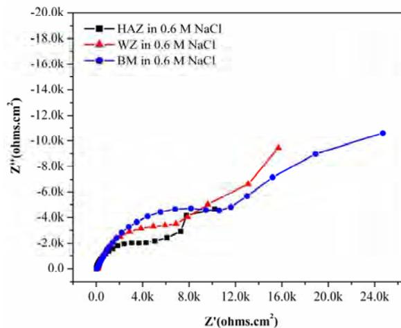
Fig.3 Nyquist plot for top surface of AA2219-T87 welded plate in 0.6 M NaCl
