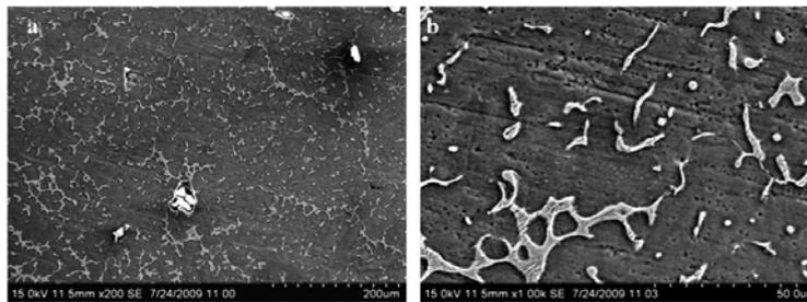
Fig. 6 SEM image of HAZ (a) Lower magnification (b) Higher magnification
