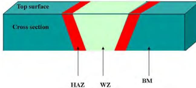
Fig.1. Locations of test specimens of Base metal (BM), heat affected zones (HAZ),weld zone (WZ)
