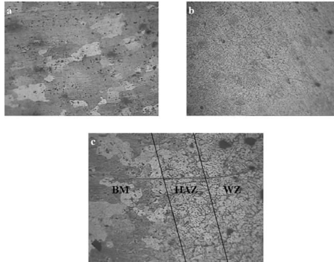
Fig.4 100X Microstructure of (a) BM, (b) WZ, (c) HAZ
