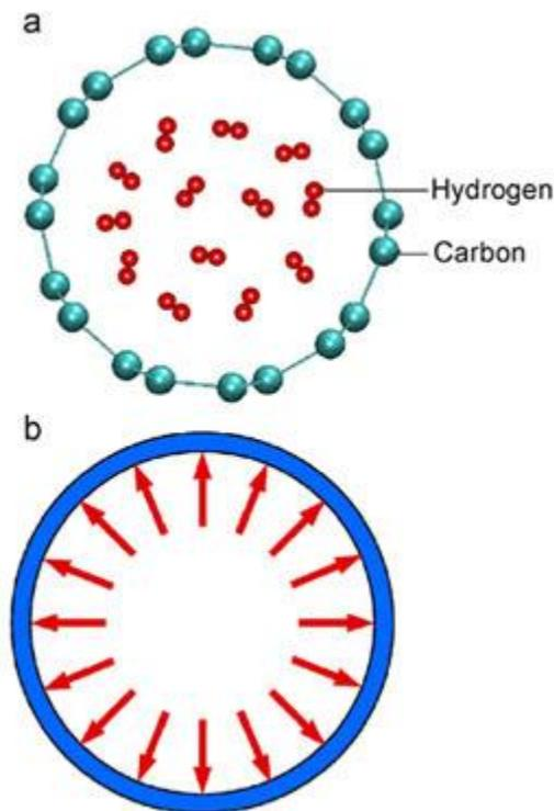
Attempts to model physisorption have lead to a study comparing analytical atomic modeling (AFEM) with a continuum model, in which the carbon tube is equated to a pressure vessel and the hydrogen stored is equated to an internal pressure. The figure to the left, from Chen et al in 2008[4], shows the analogy between the two methods (where (a) is AEFM, and (b) is the continuum model).
