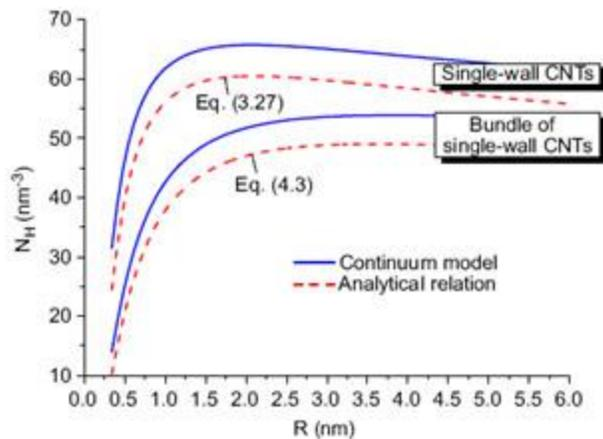
This study showed hope that CNTs could achieve the desired 18.7 molecules per nm<sup>3</sup> as mentioned earlier in this article. The figure above, from the same study[4] shows a correlation between nanotube radius and simulated storage capacity.
