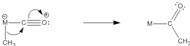
**Figure MI2.4. A migratory insertion reaction, this time forming an acyl compound.**
