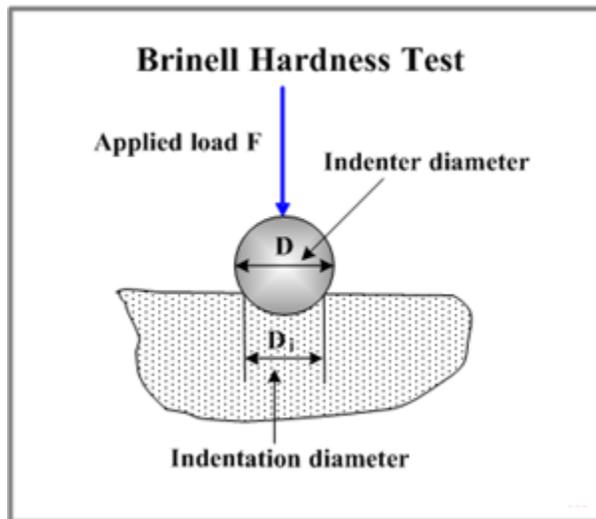
In this test a hardened steel (or tungsten carbide for extremely hard materials) ball of 2.5, 5 or 10 mm in diameter is used as indenter.
