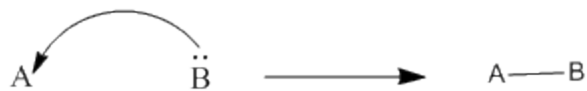
Figure AB1.1. Electron movement and bond formation in a generalized reaction. Here, atom B is donating a pair of electrons to atom A.
