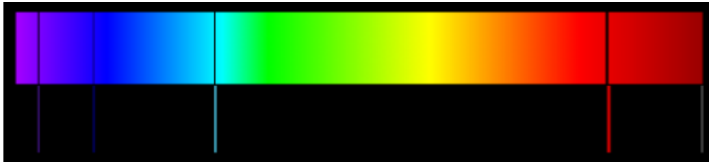
Emission and absorption spectrum of Hydrogen. Image adapted from the one by Wikimedia Commons
