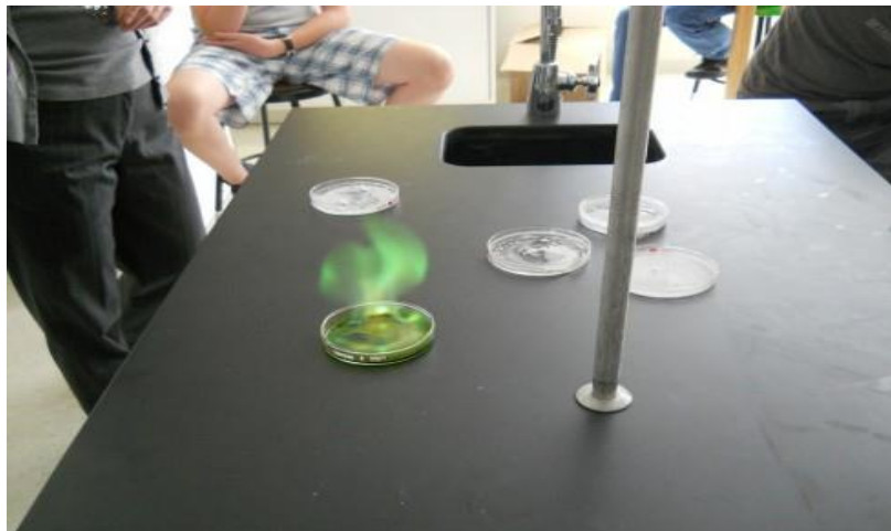
Copper burns green.
