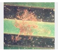
The rate of electromigration increases with temperature and has four prerequisites – a mobile metal; a voltage gradient; a continuous film of moisture; soluble ions:
