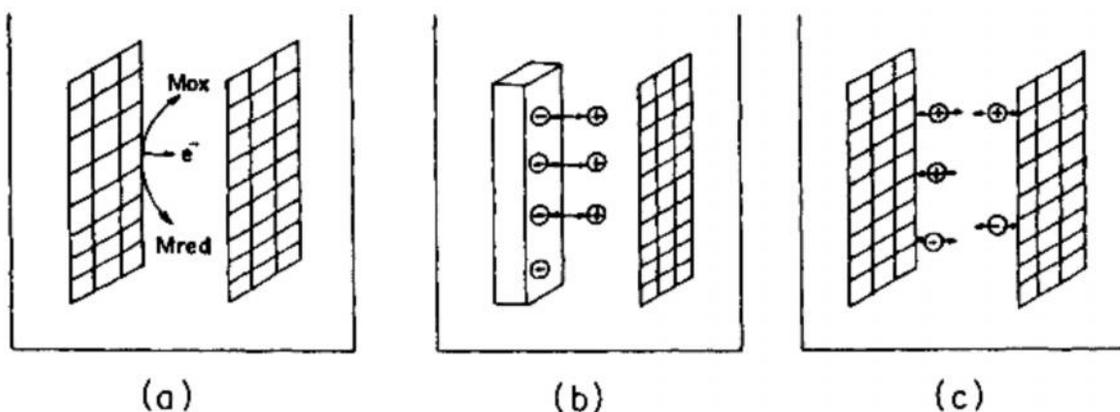
**Figure 2.** Principle of (a) amperometric, (b) potentiometric and (c) conductimetric biosensors;  $M_{red}$ , reduced mediator;  $M_{ox}$ , oxidised mediator;  $\ominus$ , anion;  $\oplus$ , cation.
