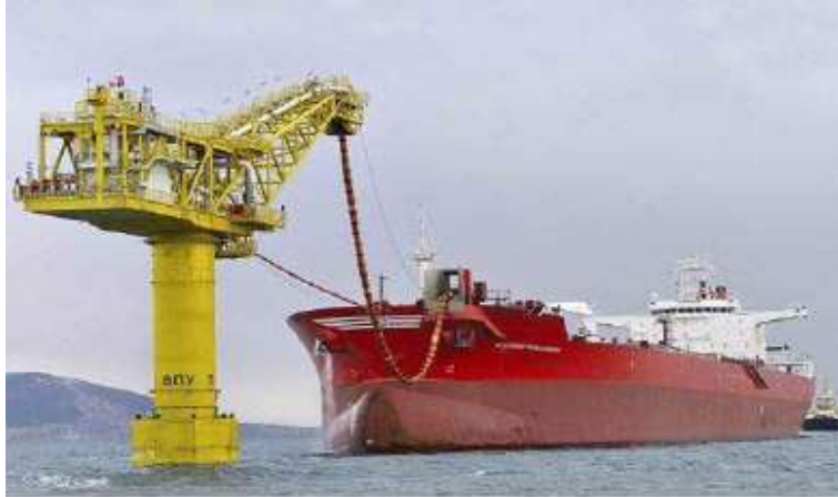
Figure 12: Example of mooring ship to SPM (courtesy of SBM Offshore)
