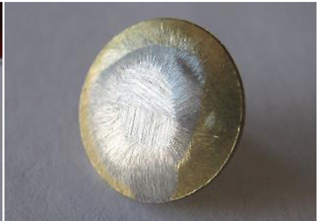
Abraded pin revealing steel
