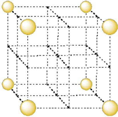
**Figure ME3.3. A simple cubic unit cell. The atoms are separated so that you can see their relationship more clearly.**
