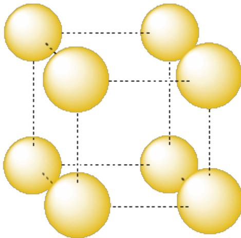
**Figure ME3.2. A simple cubic unit cell. The atoms are separated so that you can see their relationship more clearly.**
