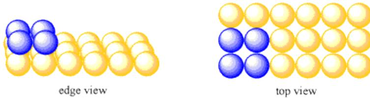
**Figure ME3.1. Adding a second layer of atoms to a simple square layer.**
