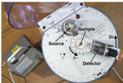
*Top view of diffractometer (Click on image to view larger version)*
