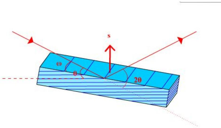
To measure the diffraction peak the sample is rotated by the offset. Now  $\omega$  is not equal to  $\theta$ . This is called an asymmetric reflection
